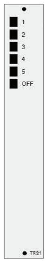
Selects which mics can be operated with remote ON/OFF switch.
